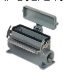
Surface mounting housing, V-TYPE series, with 1 lever, M40 x 2 cable entry, size "77.27", high construction, with plastic cover
