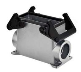
Surface mounting housing, JEI®-P series, with 2 levers, Pg21 cable entry, size "57.27", high construction
