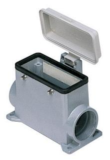
Surface mounting housing, 830V series, with 4 pegs, Pg21 x 2 cable entry, size "77.27", with plastic cover
