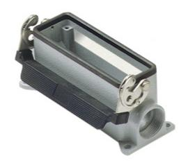
Surface mounting housing, 830V series, with 1 lever, M40  $\times$  2 cable entry, size "104.27", high construction
