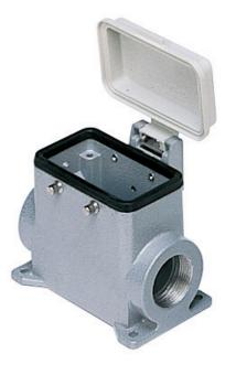
Surface mounting housing, 830V series, with 4 pegs, M40 cable entry, size "57.27", high construction, with plastic cover
