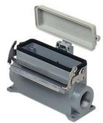
Surface mounting housing, JEI®-V series, with 1 lever, Pg29 cable entry, size "77.27", high construction, with plastic cover
