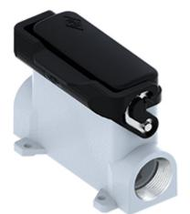
Surface mounting housing, IL-BRID series, with 1 lever, Pg16 cable entry, size "66.16", high construction, with SIMPLEX self-closing cover
