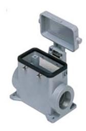
Surface mounting housing, 830V series, with 4 pegs, M32 cable entry, size "57.27", high construction, with metal cover
