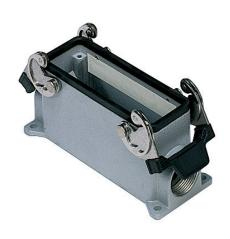
Product type Surface mounting housing Series Closing type With 2 levers Size Size "104.27" With cable entry **Cable entry** Specification High construction Technical data IP65 / IP66 / IP69 IP degree of protection **Further technical details** Operating temperature range (min, max) -40°C...+125°C
