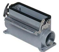
Surface mounting housing, JEI®-V series, with 1 lever, M32 cable entry, size "77.27", high construction
