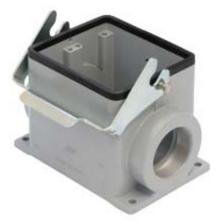
Surface mounting housing, JEI $\mbox{B-V}$  series, with 1 lever, M40 x 2 cable entry, size "77.62", with plastic cover
