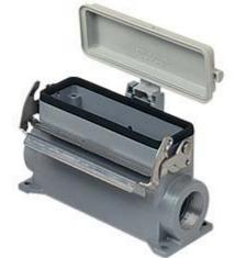
Surface mounting housing, JEI  $\ensuremath{\mathbb{B}}$  -V series, with 1 lever, Pg21 x 2 cable entry, size "57.27", high construction, with plastic cover
