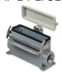
Surface mounting housing, V-TYPE series, with 1 lever, M32 cable entry, size "104.27", high construction, with plastic cover
