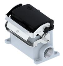
Surface mounting housing, V-TYPE series, with 1 lever, M40 cable entry, size "57.27", high construction, with SIMPLEX self-closing cover
