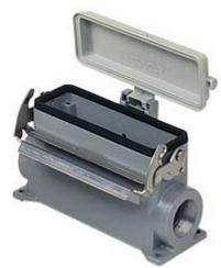
Surface mounting housing, JEI®-V series, with 1 lever, M32 cable entry, size "77.27", high construction, with plastic cover
