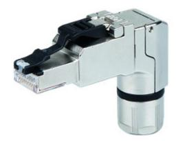
Male RJ45 connector, DTJ connectors series, angled, with metallic cable strain relief, Cat. 6A, IDC, contact coding according to T568A
