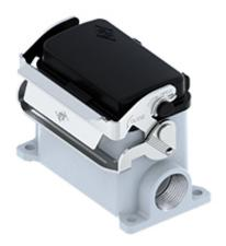
Surface mounting housing, V-TYPE series, with 1 lever, M25 cable entry, size "57.27", high construction, with SIMPLEX self-closing cover
