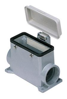
Surface mounting housing, 830V series, with 4 pegs, M32 x 2 cable entry, size "77.27", high construction, with plastic cover
