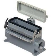
Surface mounting housing, JEI  $\ensuremath{\mathbb{B}}$  -V series, with 1 lever, M32 x 2 cable entry, size "57.27", high construction, with plastic cover
