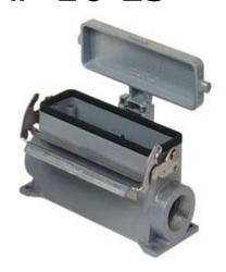
Surface mounting housing, V-TYPE series, with 1 lever, Pg21 cable entry, size "77.27", high construction, with metal cover
