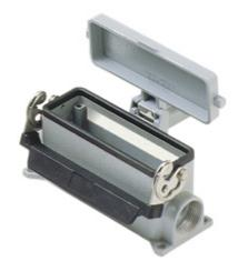
Surface mounting housing, 830V series, with 1 lever, Pg29 x 2 cable entry, size "104.27", high construction, with metal cover
