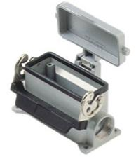
Surface mounting housing, 830V series, with 1 lever, Pg21 cable entry, size "77.27", high construction, with metal cover
