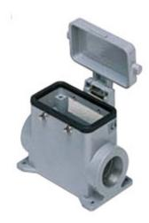
Surface mounting housing, 830V series, with 4 pegs, Pg29 cable entry, size "57.27", high construction, with metal cover
