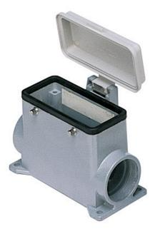
Surface mounting housing, 830V series, with 4 pegs, M40 x 2 cable entry, size "77.27", high construction, with plastic cover
