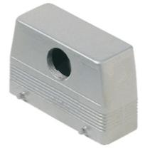
Hood, 830V series, with 4 pegs, Pg21 frontal cable entry without adapter, size "104.27", high construction
