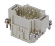
Male insert, CDS series, spring terminal connection, 9 poles + PE, 10 A 400 V 6 kV 3, size "44.27"
