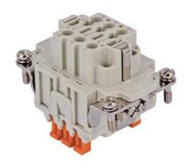
Female insert, CDSH NC series, SQUICH® spring terminal connection without tools, 6 poles + PE, 6 A 250 V 6 kV 3, size "44.27", with AutoShort NC contact element
