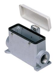
Surface mounting housing, C-TYPE series, with 4 pegs, Pg29 cable entry, size "104.27", high construction, with plastic cover
