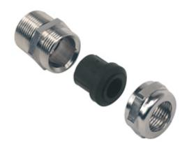
Complete cable gland, Pg16, for diameter 9,5-14 mm, 15 mm threading length
