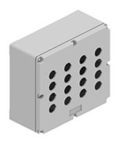
Box for control devices and signals, AC series, without cable entry, 16 holes for unit  $\emptyset$  22 mm, external dimensions 230x205x102 mm
