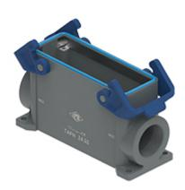
Surface mounting housing, T-TYPE /H series, with 2 levers, M40 x 2 cable entry, size "104.27", with integrated protective PE jumpers
