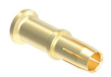
Female crimp contact, RX7 series, 70 A, turned gold plated, wire cross section 16 mm<sup>2</sup>, AWG 6 - 5, extra-flexible Class 6 conductor, HNM - High Number of Matings version
