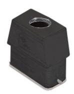
Hood, W-TYPE series, with 2 pegs, M25 top cable entry without adapter, size "49.16", high construction
