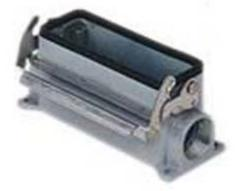
Surface mounting housing, V-TYPE series, with 1 lever, M32 x 2 cable entry, size "77.27", high construction
