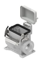
Surface mounting housing, V-TYPE series, with 1 lever, M32  $\times$  2 cable entry, size "44.27", high construction, with plastic cover
