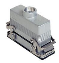
Complete connector, CSZ series, composed of 2 spring terminal connection inserts with 16 poles + PE, and bulkhead mounting housing with 2 levers and hood with top cable entry
