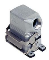
Complete connector, CSZ series, composed of 2 spring terminal connection inserts with 24 poles + PE, and bulkhead mounting housing with 1 lever and hood with side cable entry
