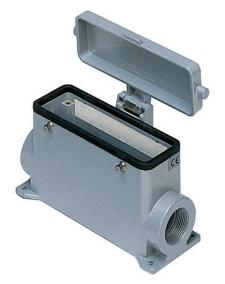
Surface mounting housing, 830V series, with 4 pegs, M25 x 2 cable entry, size "104.27", with metal cover
