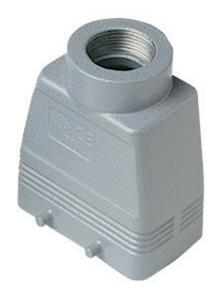
Hood, 830V series, with 4 pegs, M40 top cable entry, size "57.27", high construction
