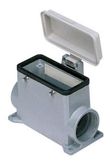
Surface mounting housing, 830V series, with 4 pegs, M40 cable entry, size "77.27", high construction, with plastic cover
