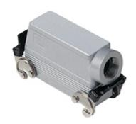
Hood, 830V series, with 2 levers, M32 side cable entry, size "104.27", high construction, without gasket
