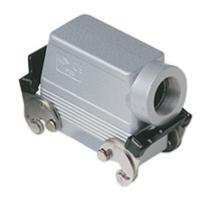
Hood, 830V series, with 2 levers, M32 side cable entry, size "77.27", high construction, without gasket
