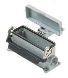
Surface mounting housing, C-TYPE series, with 1 lever, M40 cable entry, size "104.27", high construction, with metal cover
