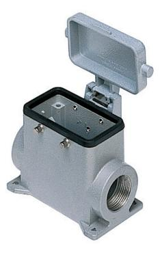
Surface mounting housing, C-TYPE series, with 4 pegs, M32 x 2 cable entry, size "57.27", high construction, with metal cover
