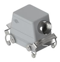
Hood, C-TYPE series, with 2 levers, M32 side cable entry, size "66.40", high construction, without gasket
