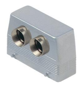
Hood, C-TYPE series, with 4 pegs, M25 x 2 double frontal cable entry, size "104.27", high construction
