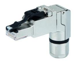
Male RJ45 connector, DTJ connectors series, angled, with metallic cable strain relief, Cat. 6A, IDC, contact coding according to T568B
