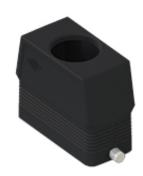
Hood, W-TYPE series, with 2 pegs, Pg21 top cable entry without adapter, size "49.16", high construction
