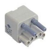
Female fibre optic connector, CXL DESINA inserts series, 2 pole fibre optics + 4 poles + PE, 10A 250V 4kV 3; 10A 230/400V 4kV 2, size "21.21", for hoods, with 4+1 CD 1.5 crimp contacts and 2 HCS fibre optic contacts
