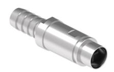
Female pneumatic metal contact, straight, hose barbs, with shut-off valve, inner diameter 10 mm
